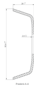
Longitudinal rail insulating spacer under the four-hole steel fishplate
